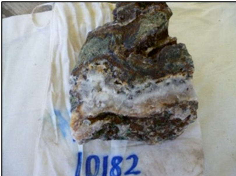
Figure 5 - Banded quartz vein with comb texture and iron oxide after sulfides at Isina Prospect
